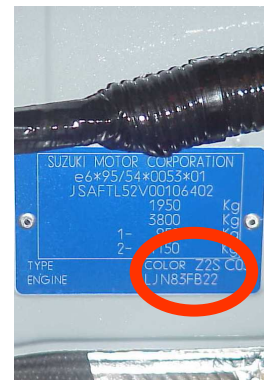
VIN PLATE SUZUKI PAINTCODE = Z2S
